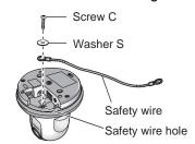
Attach ceiling plate A (included) to the camera by aligning it as shown. Secure the plate to the camera firmly.
