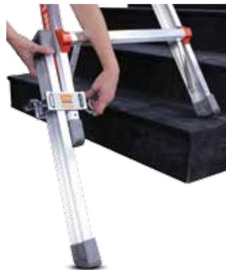
2. Slide the H-bracket onto the outer ladder leg as close to the ladder foot as possible. Insert clamp into the H-bracket and securely tighten. If the angles are not the same, remove leg clamp and rotate the channel assembly 180 degrees, and then replace leg clamp.
