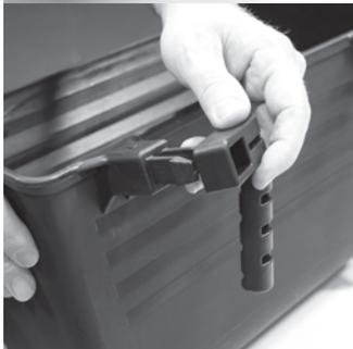
**Turn the "A" arm so the "A" is facing toward the Fuel Tank.**
