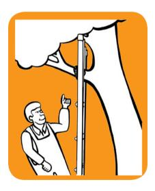
• Tying the ladder to a firm support near the top will help to prevent slipping or tipping.
