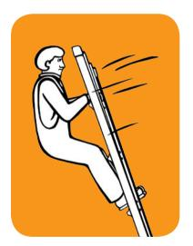
A ladder placed too close may tip over backward. Place the bottom one foot out for each four feet of height.
