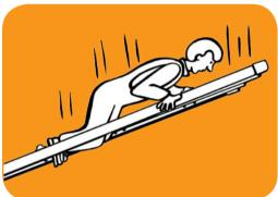
Set the ladder at the proper angle; when a ladder is too far out it may slip out at the bottom.
